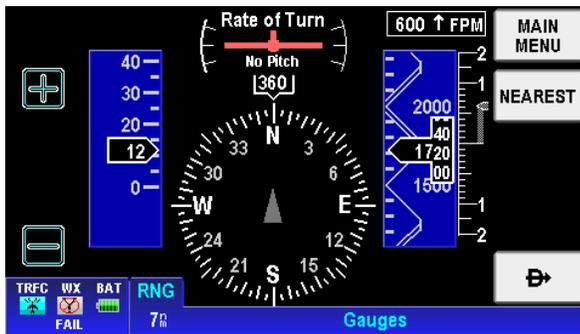
A new feature, the AV8OR Portable Glass Panel, has been added as an option from the main menu. This page simulates a modern, glass panel PFD. The instruments are based on GPS input ONLY. Therefore, the AV8OR Portable Glass Panel displays Rate of Turn, Ground Speed, GPS Altitude, Vertical Speed and a Compass Rose integrated with the aircraft flight plan display.
